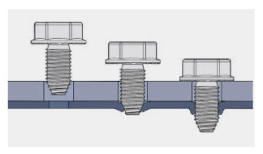
Framo is assembled via thread forming screws. The non-cutting cold formed threads of the screw form their own threads to pilot holes of the perforated Framo profiles. The low thread forming torque and resulting high clamping force, offers a superior process-reliable shake-proof fastening. The thread forming screws are removable and can be used again.
